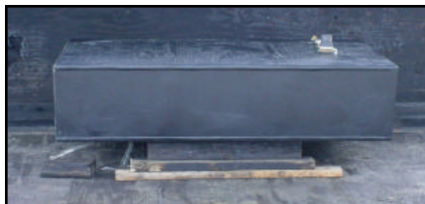
Figure 2: view of tank following fire test
