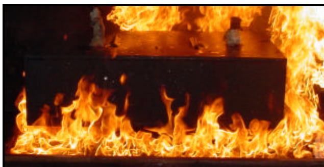
Figure 1: view of tank undergoing fire test
